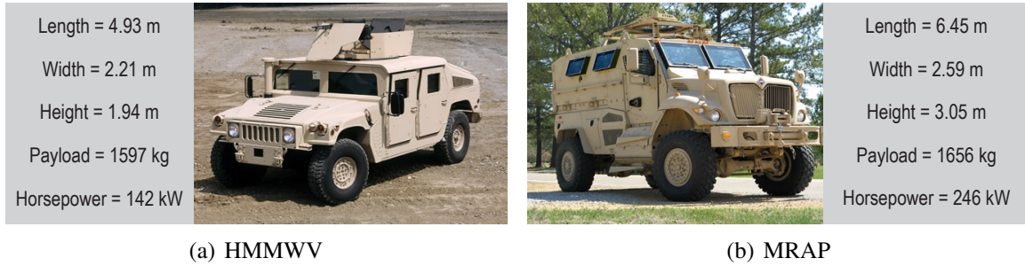
Figure 3.1: Two current military ground vehicle options and their associated capabilities (data from www.amgeneral.com , www.defense-update.com , www.militaryfactory.com , and www.navistardefense.com )
